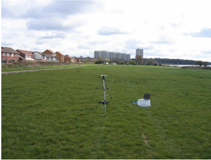
FIGURE 4.18: Photo showing LOS testing location 0.0 m - 250.0 m. Initiator node placed on tripod stand and interfaced to laptop computer for data extraction and logging. Responder moved across field with unobstructed signal path. March 2007.
